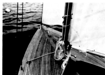
Details like the deck planking ribbed into the king plank, and the coaming breast hook are pleasing to the eye, after the whole boat has been taken in.
